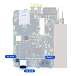
We also recommend you remove the coin cell battery and dispose of it in an environmentally friendly way.
